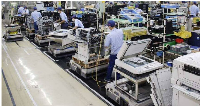
Recycle line (disassembly and assortment processes)
