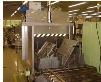
Automatic shower washer that cleans accessories
